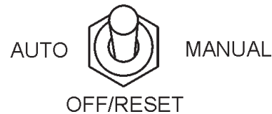
Figure 56. MPEC Control Switch (Off/Reset)
