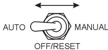
Figure 55. MPEC Control Switch (AUTO)
